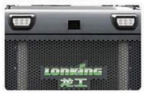
Equipped with LED tail lights and camera.
