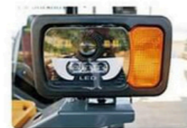
LED lens lamp, energy-saving, transparent, and long service life.
